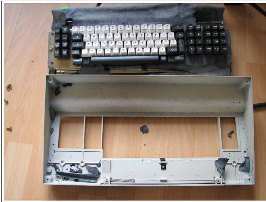
Figure 2: 3278 keyboard with top half of case removed (image courtesy of webwit )
